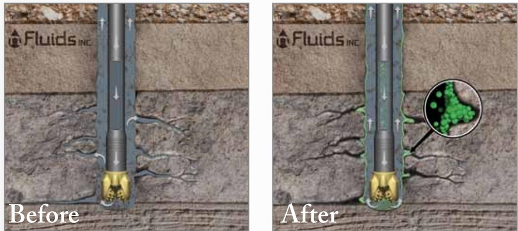
nFluids Inc. has had impressive lab results, and the technology demonstrates the ability to reduce drilling fluid loss by up to 90% (as per API test standards).
